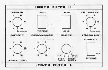
The filters in the FILTER/ADSR path may be used to create various filter responses. The Upper Filter is a lowpass resonant filter with choice of 12dB or 24dB cutoff slope.
